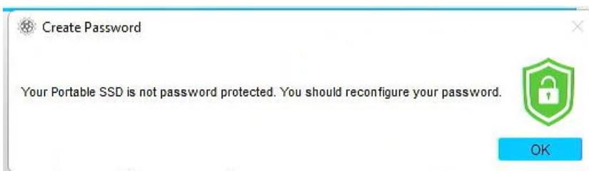
If this pop-up is displayed, click "OK" button to close the pop-up window, change the USB port to which the device is connected, execute "Remove Password" operation, and then perform "Set Password" operation again.
