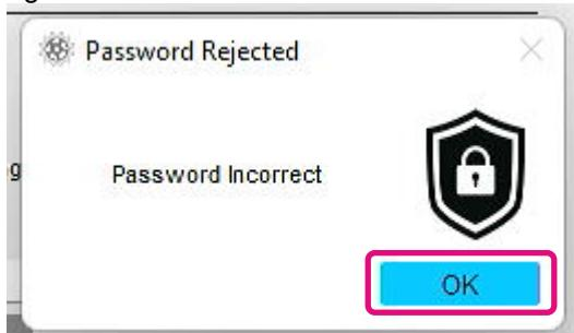
If you enter the wrong User Password five times in a row, the following will appear on the SSD Utility. In this case, please disconnect the target device from the USB port safely and reconnect it to reset the retry counter. And then, please execute "Unlock device" again.
