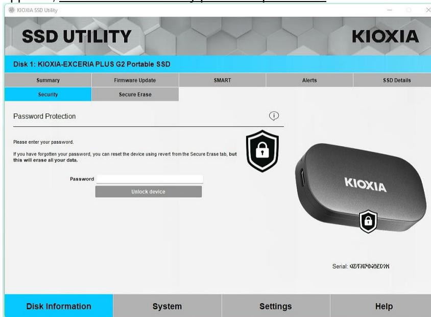
If the black shield icon does not appear here, select "KIOXIA-EXCERIA PLUS G2 Portable SSD" and select "Security" tab. If "Remove Password" button appears even though you have not "Unlocked the device" as shown below, the password protection may not be set correctly. In this case, please click the "Remove Password" button to remove the passwords, and then try "Set Password" again.
