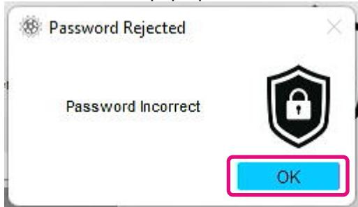
If you enter the wrong Password five times in a row, the following will appear on the SSD Utility. In this case, please disconnect the target device from the USB port safely and reconnect it to reset the retry counter. And then, please execute "Unlock device" again.
